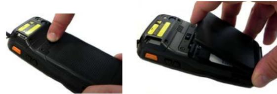
2. Open the card slot and insert the microSD card with the written part downward
