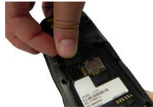
3. Shift the microSD card to the right to lock it into the cardholder; close the card slot:
