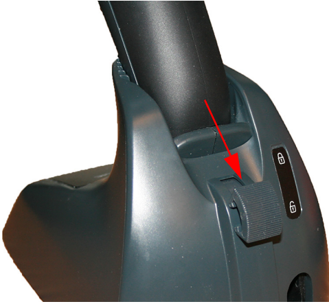
Figure 1. Lock lever disengaged
