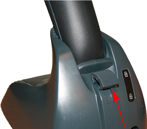
Figure 2. Lever in locked position
